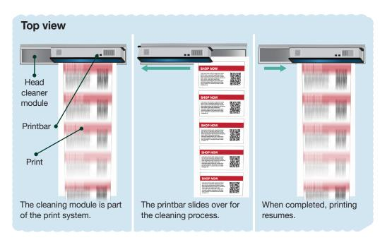
The cleaning/capping module is specially designed with precision engineered components to help maintain optimal image quality throughout the life of the 46kUV product. The module is typically run once per shift, and at the touch of a button, cleans the printhead nozzle plate to address issues arising from misdirected or lost nozzles.
